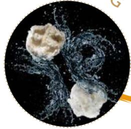
This is the link between the natural fibre and the product, and as such, it requires great respect, delicacy and attention to every detail. The water is the main factor in this process: after washing the freshly sheared fleece, the next step is to remove every impurity.
