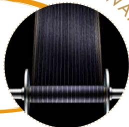
Warping is a wonderful exercise in geometry, where vertical threads of the fabric will become part of a complex weave. Every single thread and hundreds of spools are simultaneously monitored by sensors until the warp is wound onto a cylinder, called a beam.
