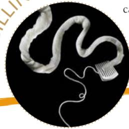
The wool is combed a number of times to achieve parallelity and the short fibres are discarded. The semi-finished product is called top and its quality is extremely important to guarantee the durability of the final fabric.
